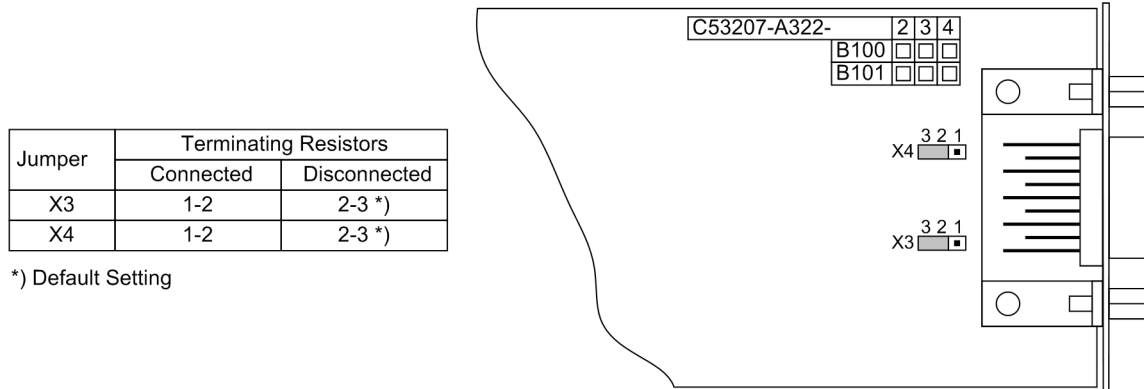
Figure 3-11 Position of the plug-in jumpers for the configuration of the terminating resistors at the Profibus (FMS and DP), DNP 3.0 and Modbus interfaces
